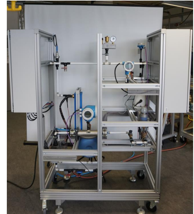
Photo of the laboratory test facility with the ohmic heating reactor, sensors and actuators and the electric boxes.
